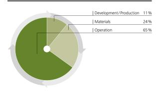
The energy consumed while an elevator is in service (operation phase) accounts for two-thirds of its environmental impact.
