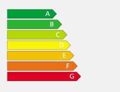
The measurement standard is VDI 4707 established in March 2009 by the Association of German Engineers. Energy efficiency classification can vary depending on elevator configuration.
